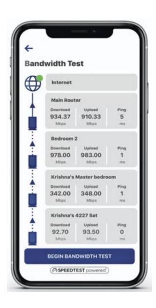
To run a bandwidth test simply select the "Begin Test" button at the bottom of the screen. The speed test will first run between the Blast router and the Internet and then will conduct a speed test between any access points and the Blast router. Results will show as a notification update at this location, and on your main dashboard.
