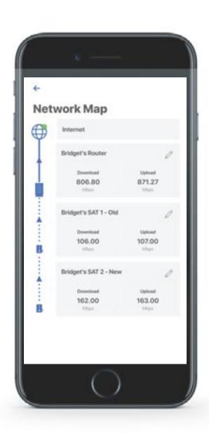
From the dashboard you can select Network Map from the bottom-righthand side of the screen. This will show any GigaCenter, Blast, or access point units connected in your network.
